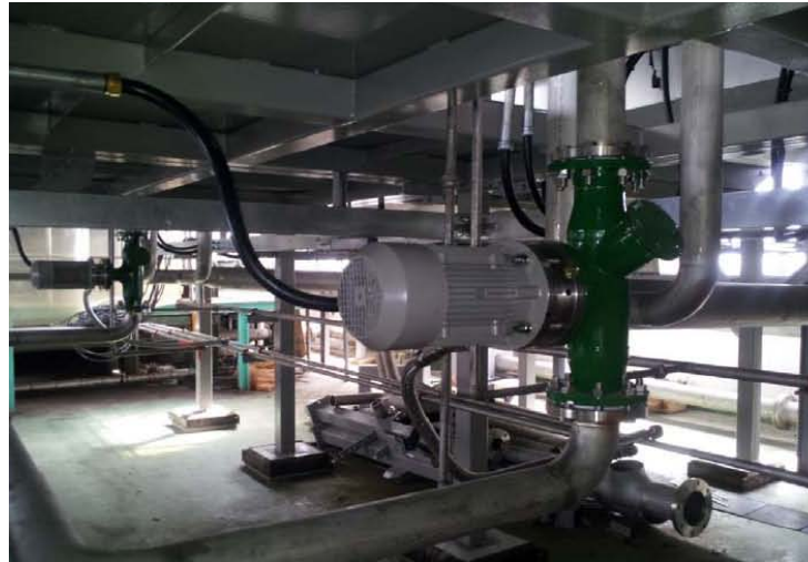
MD Screw Press (Ind. complex WWTW)
